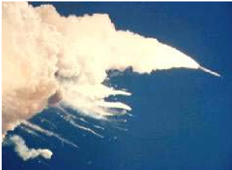
Figure 2.3 – Challenger immediately after the explosion of the SRB.
