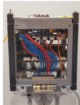
Figure 10: Many cable harnesses routed throughout GT-1 spacecraft
