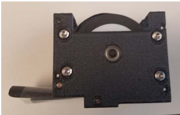
Fig. 10: Assembled boom deployer with fully stowed boom.
