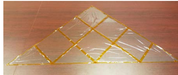
Fig. 14: CP1 sail prototype with kapton ripstops.
