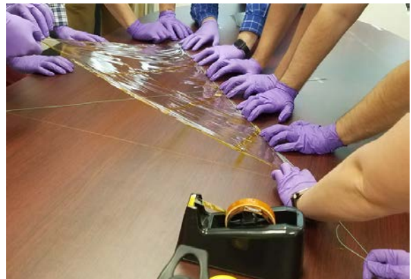
Fig. 15: Folding process. Note the green Teflon wire used to define the folds.
