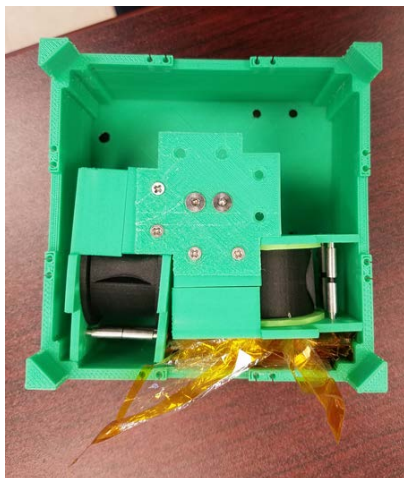
Fig. 17: Fully folded CP1 sail quadrant in the allocated volume of a 3D printed prototype
