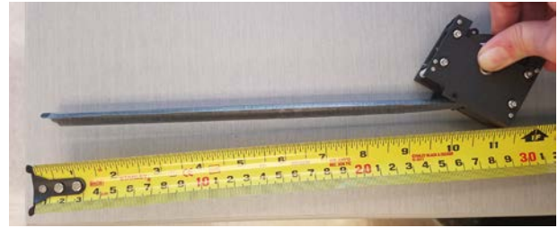
Fig. 11: Deployer held at the last point where it will free deploy
