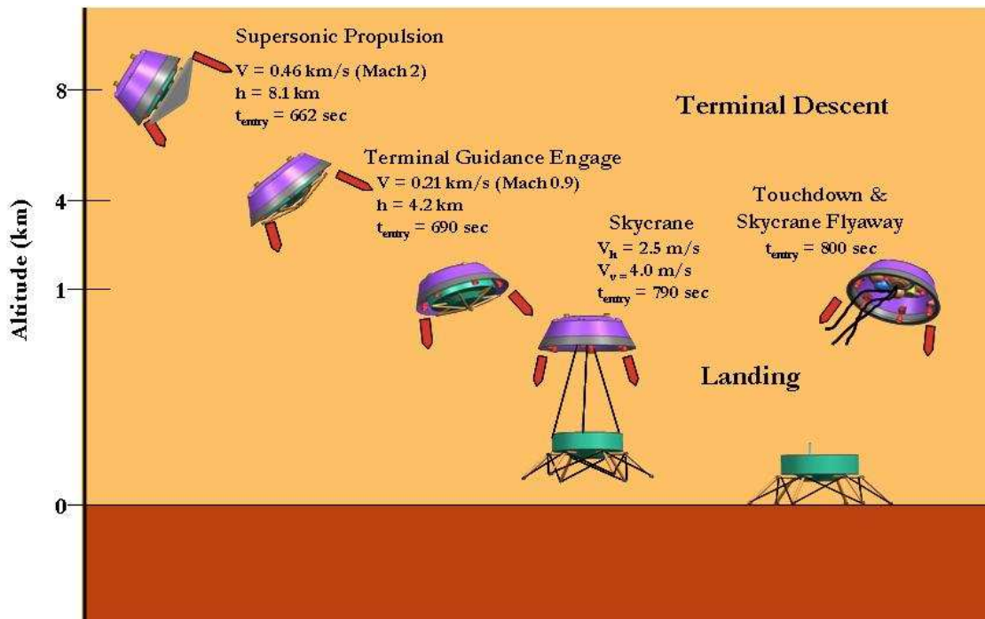
Figure 3: Nominal Descent and Landing Sequence Timeline
