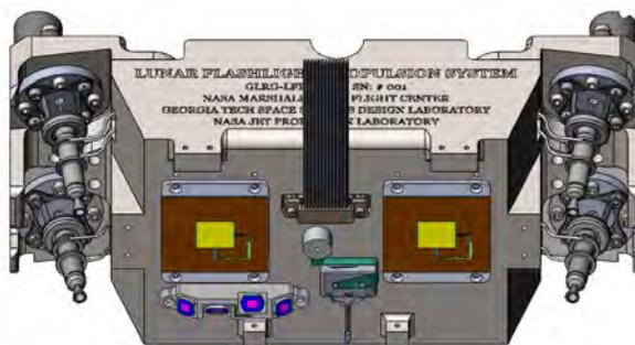
**Fig. 10** Iso-view of the muffin tin showing a few of the spacecraft electronic components connected to the +Z face of the muffin tin. The angled walls of the muffin tin near each thruster are also shown.
