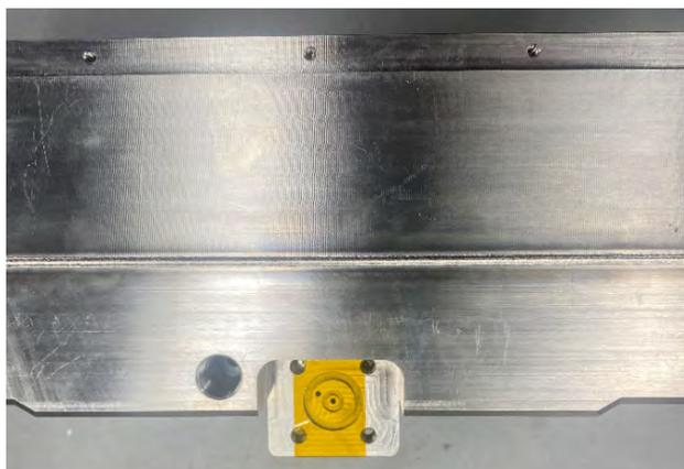
**Fig. 14 EB weld of the pathfinder tank assembly**
