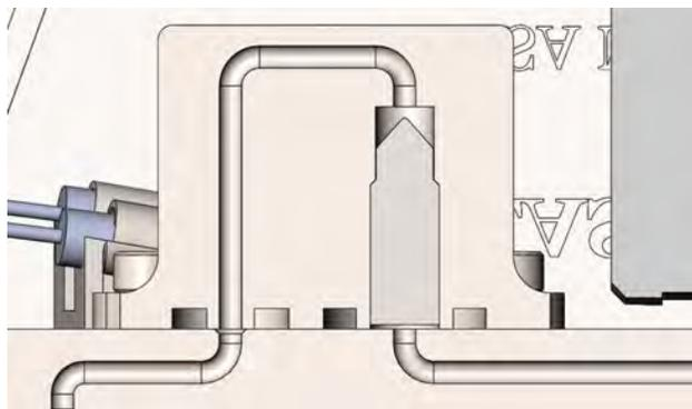
**Fig. 9** Section view of the recirculation loop passing through the recirculation block
