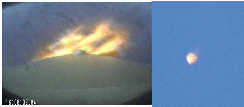
Figure 2 - Imagery of first SpaceX SRP event from onboard camera (L); ground imaging (R).
