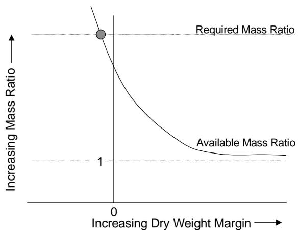
Figure 10 – Dry Weight Margin Sizing Method
