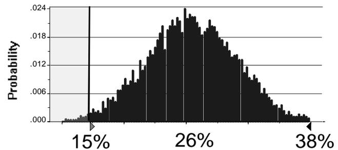
Figure 12 – All-Rocket SSTO Dry Margin Distribution
