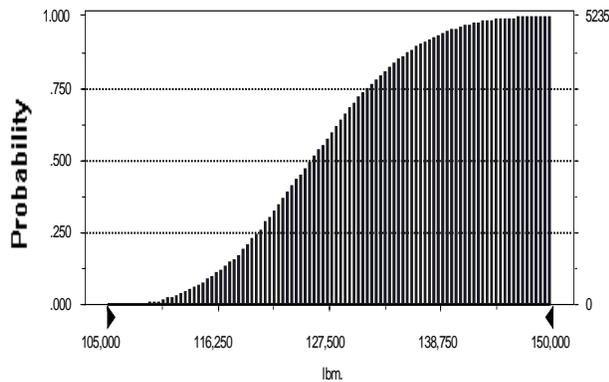
Figure 6 – All Rocket SSTO Dry Weight Cumulative
