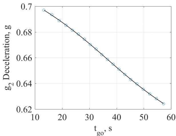
**Figure 2. Jettison  $t_{go}$  Curve Fit for Earth Aerocapture.**
