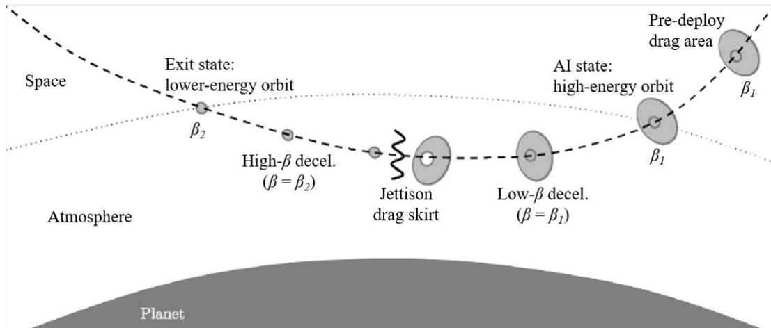
**Figure 1. Single-Event Drag Modulation Diagram<sup>6</sup>.**
