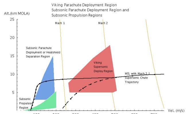
Figure 14: Supersonic Parachute Deployment Region, Subsonic Deployment Regions.
