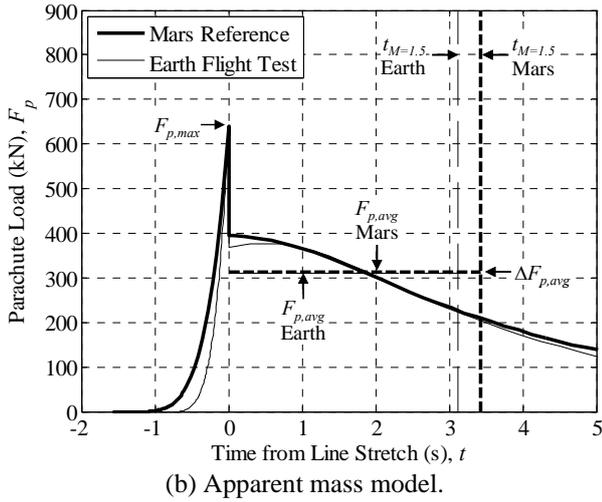
Fig. 4. Parachute load curves for  $\gamma_{Mars} = -30$  deg.
