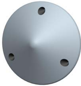
Figure 5. Example of a Peripheral Retropropulsion Configuration
