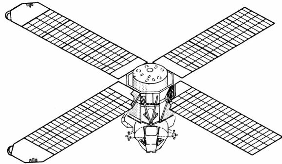
**Figure 4. Lunar-Module-Based Apollo Telescope Mount Design dated April 1968.<sup>20</sup>**
