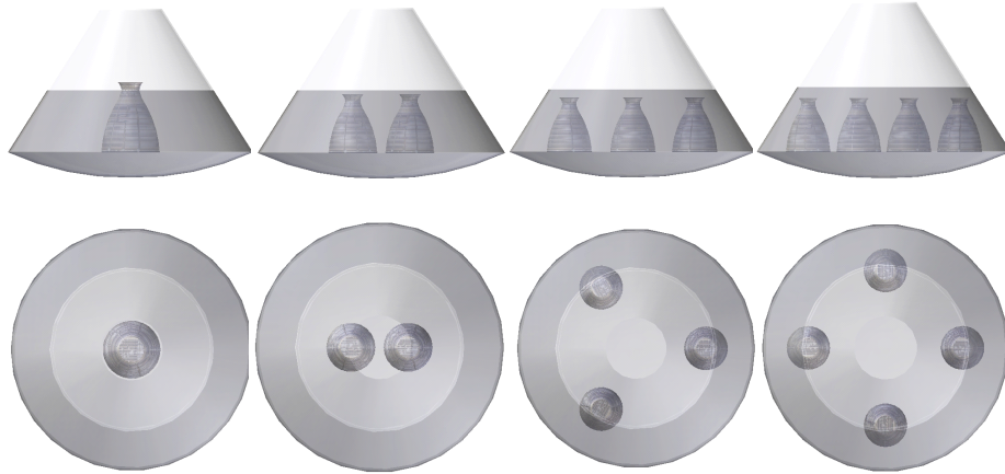
Figure 6: Engine configuration options for 10 m diameter vehicle.
