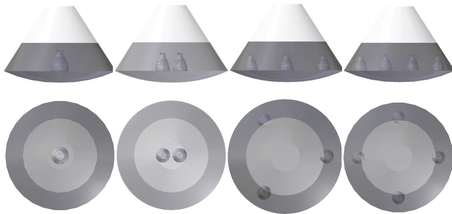
Figure 7: Engine configuration options for 15 m diameter vehicle.
