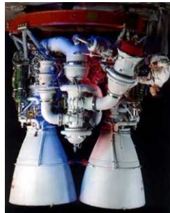
Figure 9. RD-180 Engine Design Specifications.
